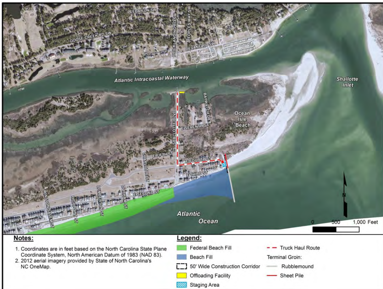
Figure 6. Location of the terminal groin and associated beach fill located on the eastern portion of Ocean Isle Beach
